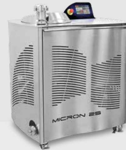
Ball mill designed for refining the product.
